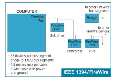
tion of the two. Each cable segment can be up to 5 meters in length. The cables have four wires, one pair for signal and one pair for power and ground. The connectors are keyed to prevent them from being plugged-in incorrectly.
